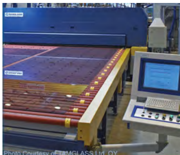
Fig. 13: From the molten state through to the cooling process, continuous temperature monitoring ensures that glass retains its properties as it travels through the manufacturing process, here the tempering of glass sheets
