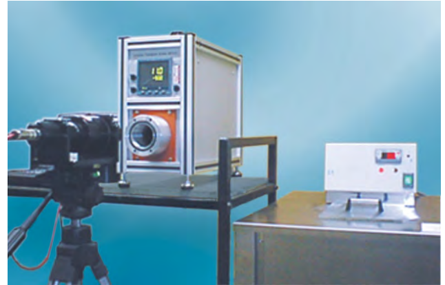
Fig. 24: Calibration of a black body using a transfer standard pyrometer, Raytek TRIRAT LT
