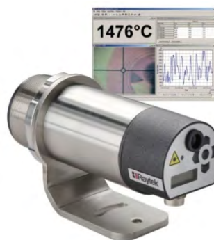
Fig. 18: Pyrometer featuring a variable distance setting – Raytek MM series with variable focus. The variable focus can be controlled manually on-site or remotely via the digital interface. Among others a video camera is used as a aiming device precisely marking the spot also when the measurement distance is changed.
