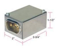
Enclosure box with EHDR-1001 cup assembly and jumpers to attach connector to screw terminals. Use with plug type 900. Mount box on mica, ceramic, or MIPlus band heaters or mica strip heaters to cover exposed screw terminals and wiring. For use on **Standard T3**
