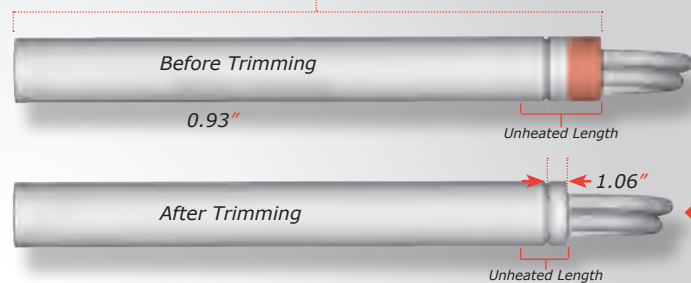
Heater size at Maximum Length Tolerance ( ALL cavity must be trimmed). 31.86"
