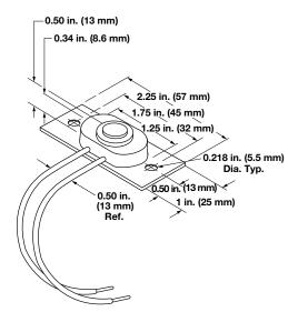
**Note:** For direct control of air temperature as is required in enclosure heating applications, specify thermostat model number ST-207E. This is a modified ST-207 mounted on <sup>1</sup>/<sub>32</sub> inch thick G-10 circuit board with the thermostat's metal cap exposed to sense air temperature.
