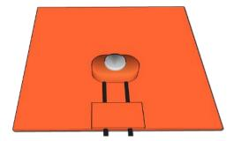
Air sensing thermostats are mounted to sense the temperature of the ambient air. They are commonly used with enclosure heaters when the air temperature is more important than the heater temperature. Air sensing thermostats can be added to stock enclosure heaters and standard stock heaters. They are available in the same temperature ratings as the surface sensing thermostats.
