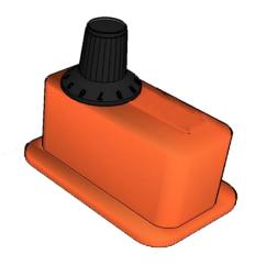
Adjustable thermostats can only be used to sense part temperature. They are often used with drum heaters but can also be used with standard heaters. Temperature adjustment range is 25°F to 330°F.
