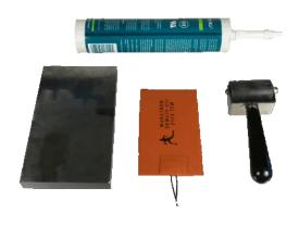
Field applied adhesive is more difficult to apply than PSA, but if done properly produces a superior bond. We can supply a room temperature curing RTV rated to 400°F. After applying a thin film between the heater and the surface, a roller should be used to remove all air bubbles, then allowed to cure for 24 hours.
