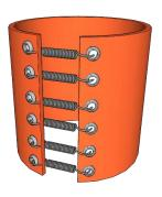
**Springs and grommets** are spaced about 2" apart. Each end of the spring is attached to a grommet securing it to the cylinder.
