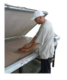
Factory Vulcanizing is the best method to bond the heater to your part. Send your part to Phoenix Thermal Supply and we will have our factory vulcanize the heater directly to your part in a vacuum
